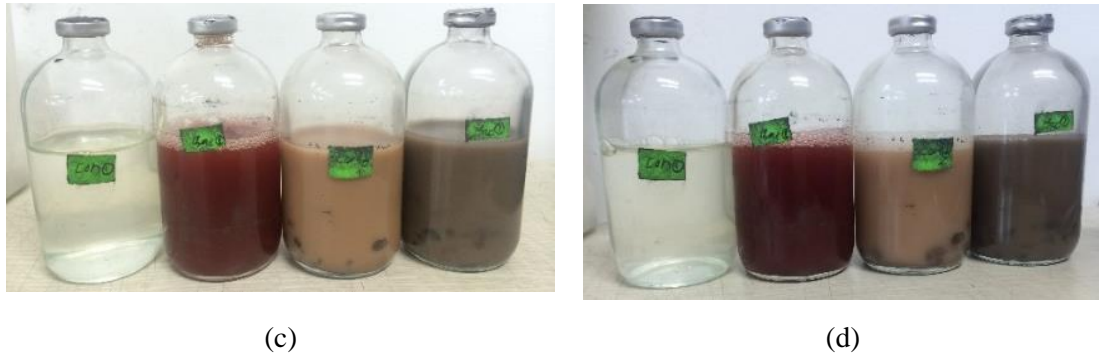
Fig. 6. Photographs of Specimen Bottles using 27s Medium, Bacteria, and Ceramic Aggregates According to the Time, with Bottles Aligned Horizontally before Shaking. The Heights of the Bottle Contents were Fixed. From the left: 100 mL medium only; 95 g ceramic aggregate and 45 mL medium; 100 mL medium and 0.5 g/L bacteria; 95 g ceramic aggregate, 45 mL medium, and 0.5 g/L bacteria. Each bottle initially contained 26 cm 3 CO 2 . (a) Immediately after inoculation, (b) 3 d, (c) 5 d, and (d) 7 d after inoculation
