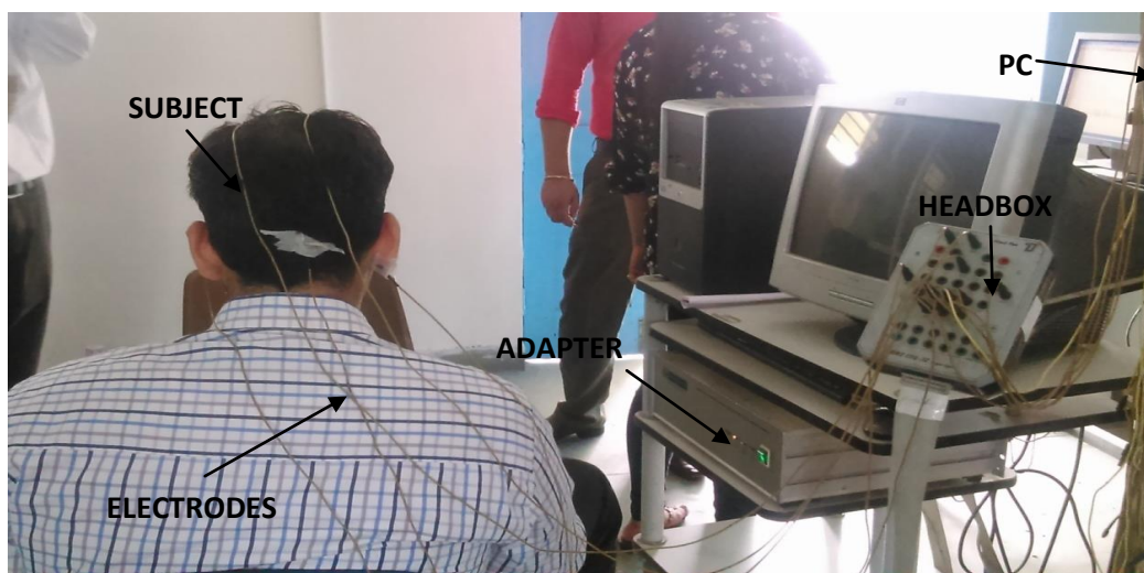
Figure 6. Experimental Setup for EEG Acquisition
