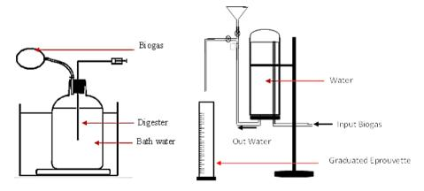
**Figure 1. Experimental Digester**
