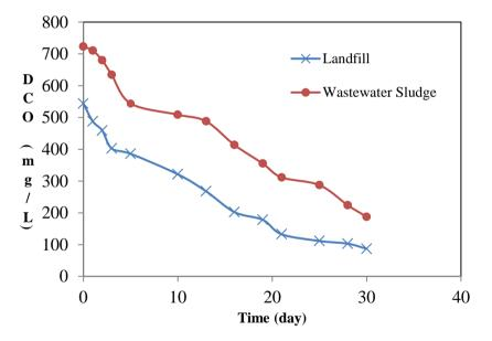
Figure 4. Variation of the COD of the Two Substrates Digestion
