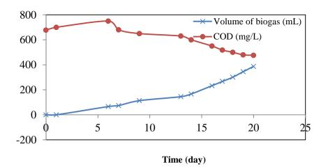
Figure 2. Anaerobic Digestion of Organic Matter from Landfill Wastes
