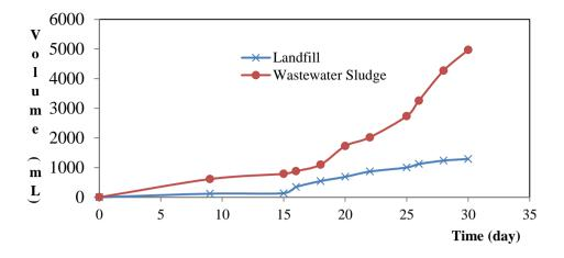
Figure 5. Biogas's Volume of the Two Substrates Digestion
