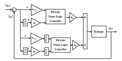
Figure 21. Design PID like Fuzzy Controller
