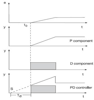
Figure 6. Ramp Response of a PD Controller
