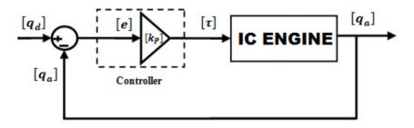
Figure 4. Block Diagram of Proportional Controller
