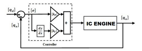
Figure 5. Block Diagram of PD Control of IC Engine
