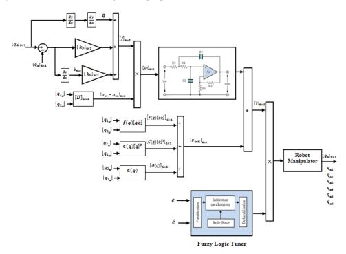
Figure 6. Block Diagram of LPF Fuzzy Computed Torque Controller
