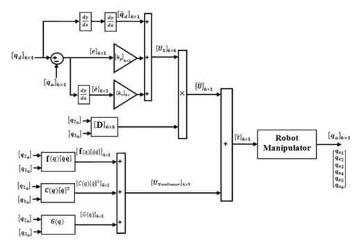
Figure 1. Computed Torque Control: Continuum Robot Manipulator
