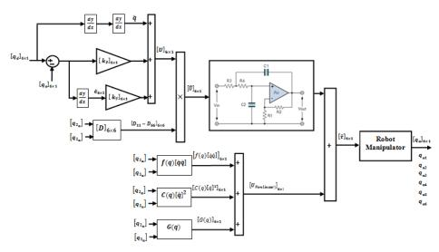
Figure 5. LPF Computed Torque Controller
