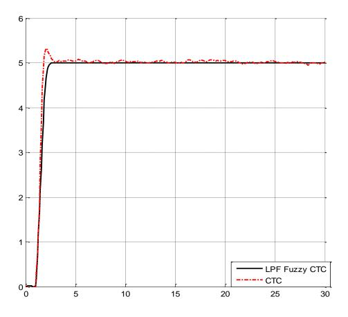
Figure 8. Power of Disturbance Rejection: LPF Fuzzy CTC and CTC
