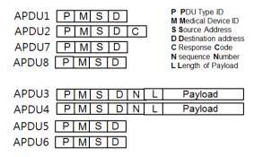
Figure 4. Application Protocol Data Unit Format
