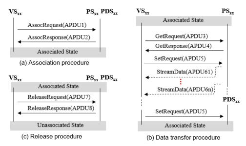
Figure 3. Application Protocol for Data Transfer
