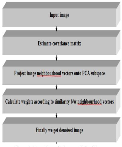
Figure 2. Flow Chart of Proposed Algorithm
