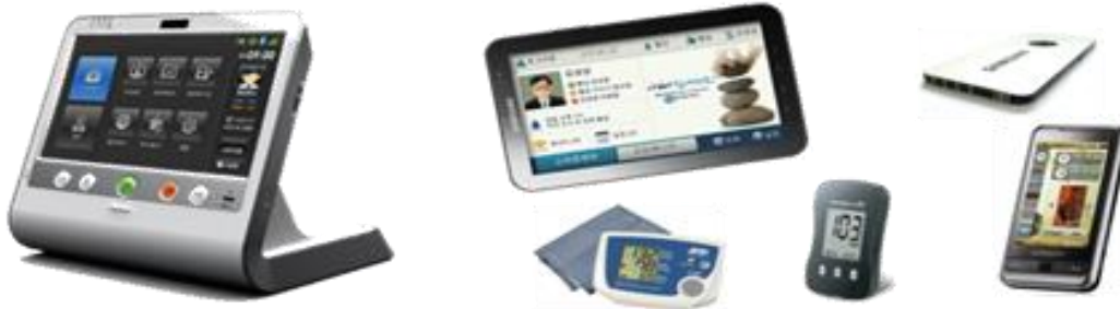
Figure 1. Dedicated Terminal-based Fixed Gateway (Left), Tablet PC-based Mobile Gateway (Center), Smartphone-based Mobile Gateway (Right)
