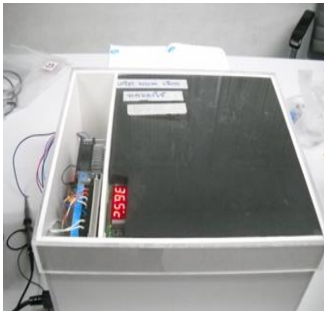
Figure 4. The Top View of the Proposed Blood Warmer Box with the Electronics and the Blood-Warming Mechanisms on the Left and Right Chambers, Respectively. During Operation, the System is Covered with EPDM and an Acrylic Top Cover to Retain the Heat
