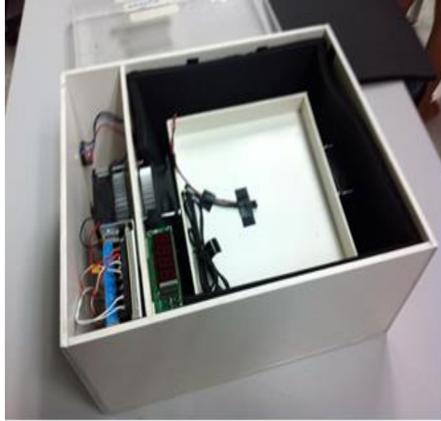
Figure 5. The Top View of the Blood Warmer System without the EPDM and Acrylic Top Cover. The White Tray is the Shaker on which a Blood Bag is Placed
