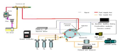
Figure 1. Schematic diagram of experimental apparatus
