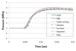
Figure 8. Pressure diagram of BD20 (P<sub>inj</sub>=100MPa)
