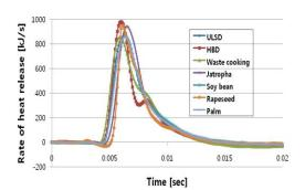
Figure 9. Heat release rates of BD20 (P<sub>inj</sub>=100MPa)
