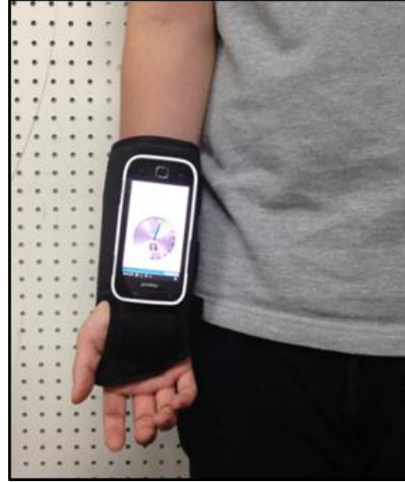
(b) Registration of the accelerometer sensor and radius bone coordinate system
