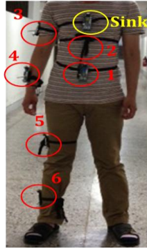
Figure 5. Locations of sink node and sensor nodes on the body
