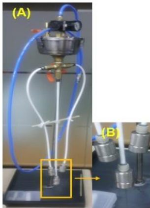
Figure 5. Picture of preparing equipment; (A) manufacturing equipment, (B) magnified needles (diameter: 0.5mm)
