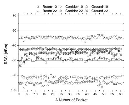
Figure 10. RSSI Values of the Back for Different Experimental Areas
