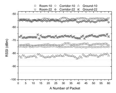
Figure 9. RSSI Values of the Stomach for Different Experimental Locations
