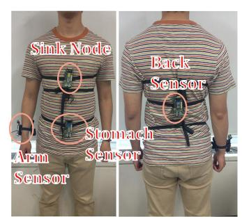
Figure 6. Sink Node and Sensor Node Deployment on the Body
