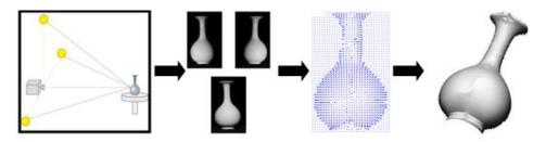
Figure 1: Illustration of a basic photometric stereo capture mechanism. From left: experimental arrangement, raw images, estimated surface normals, recovered depth. The algorithm in [4] was used here to calculate depth from surface normals.
