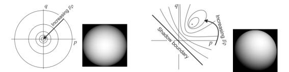
Figure 5: Solutions to (5) for p and q. The left-hand example shows the case where  $p_s = q_s = 0$ , while for the right-hand case,  $p_s = q_s = 0.5$ . The rendered images show a Lambertian sphere illuminated under these particular light source directions.
