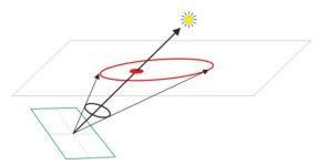
Figure 6: Representation of the solution to (5) as a conic section (in this case an ellipse). The apex of the cone lies at the point on the surface, while its axis lies along the light source vector.
