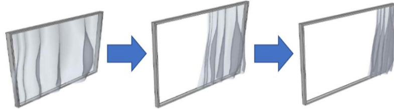
Figure 2. Concept of curtain-type aircap module attached to windows
