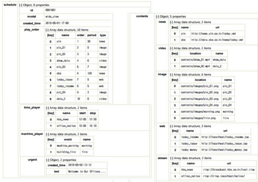
Figure 4. The Schedule Structure for a Multi Content Service
