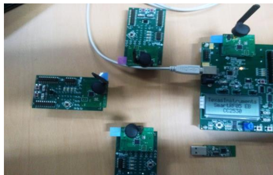
Figure 3. 6LoWPAN Home Nodes based-on TI CC2530
