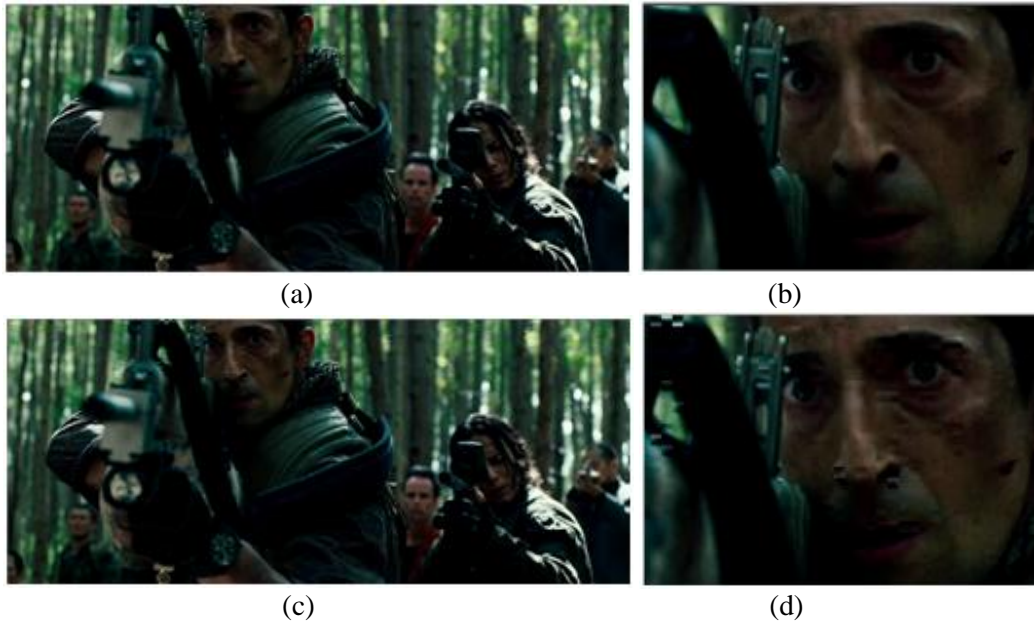
Figure 5. Any frame of (a),(b) normal recovered video after K-EM and K-DM and (c),(d) recovered video with the blocking artifacts because of recovery error by re-hiding of the random watermark. ((a),(c) : 25% scaled version of original resolution, (b),(d) : Magnified version of any region)
