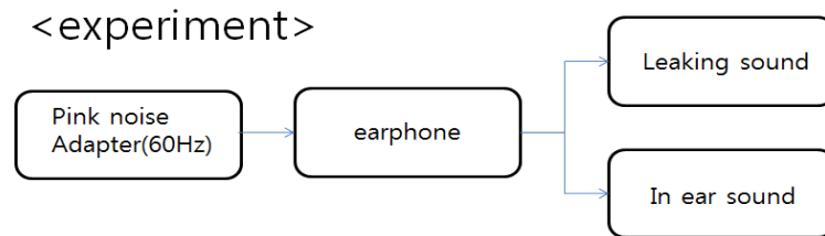
Figure 3-2. Experiment of Leaking Sound
