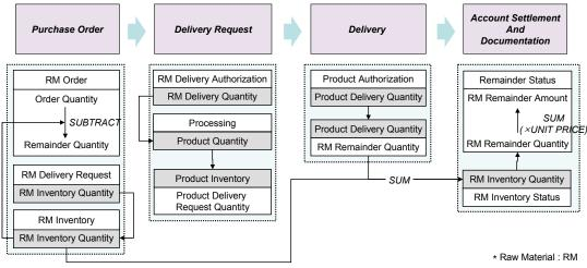
Figure 5. Dataflow in System
