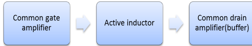
Figure 3. Block Diagram of Three Stages LNA[3]
