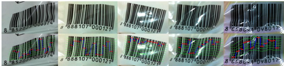
Figure 9. Test Results on Five Different Deformed Barcodes that are all Successfully Decoded
