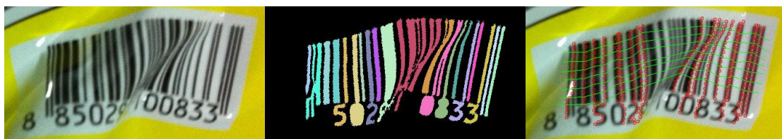
Figure 10. High Degree of Bars Merging in the Middle Part of the Barcode Causes the Algorithm to Miss Some Elements
