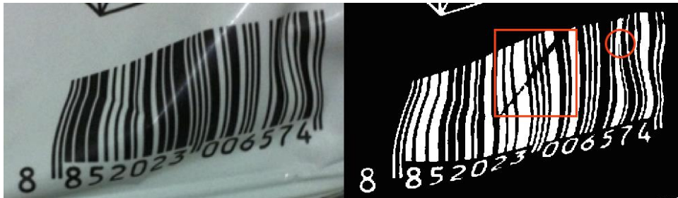
Figure 1. Example Deformed Barcode on a Wrinkled Snack Bag (left). The Barcode is Binarized Using a Simple Threshold, Showing Splits (framed by the red square) from Light Reflection, and Merged Lines (marked by the red circle) from the camera viewpoint (right)
