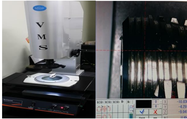
Figure 1. Implant Size Test Using Non-contact Optical Measurement Instrument
