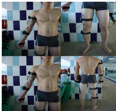
Figure 2. Attachment Placement of Gyro Sensor & Electrode
